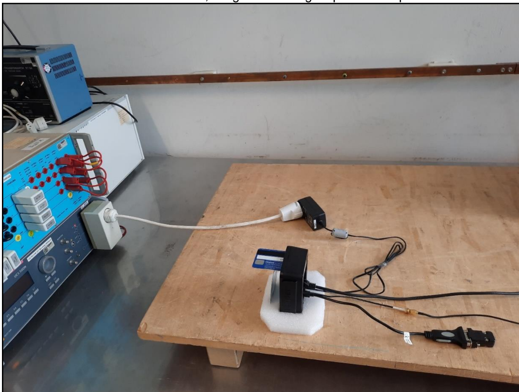
Photo 12: Burst, Surge and Voltage dips test setup
