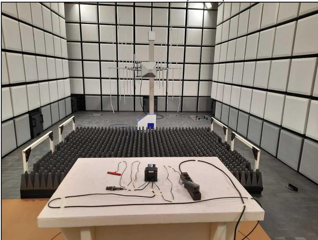
Photo 4: Radiated immunity test setup
