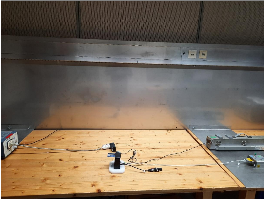
Photo 7: Conducted emission test setup
