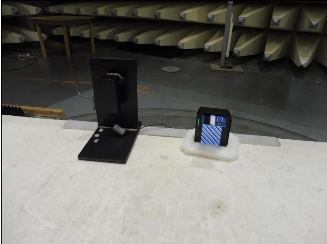
Photo 1: Radiated Emission test setup
