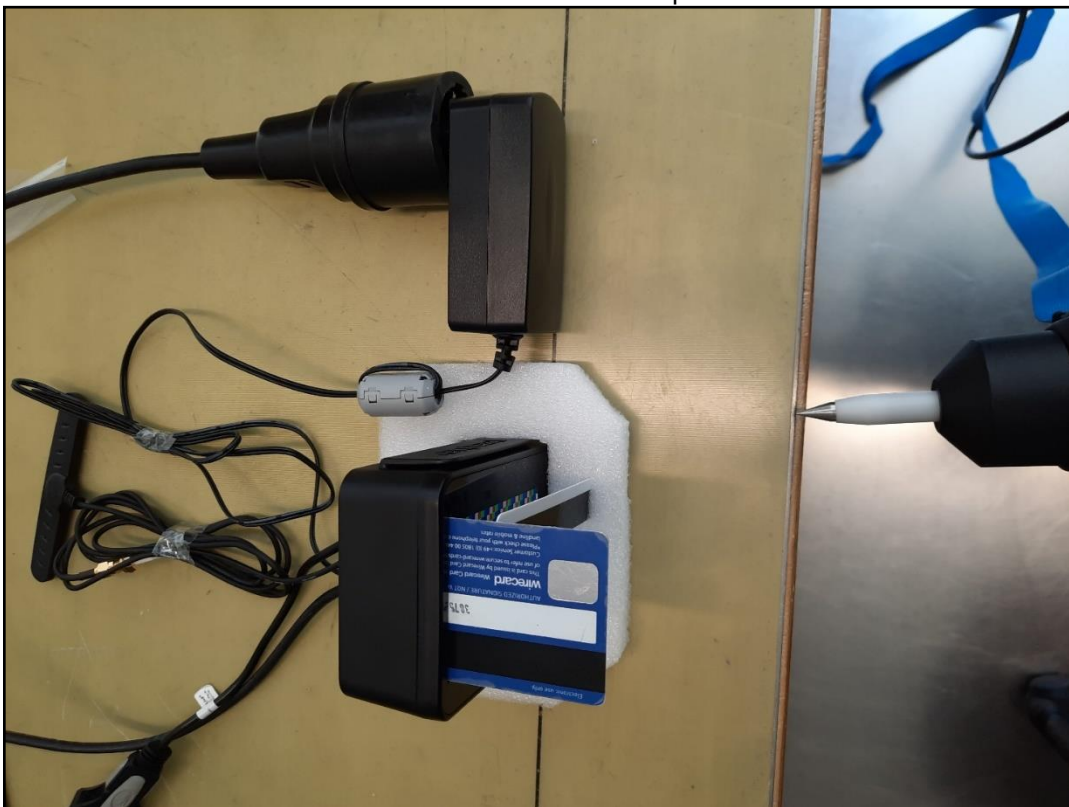
Photo 16: ESD test setup
