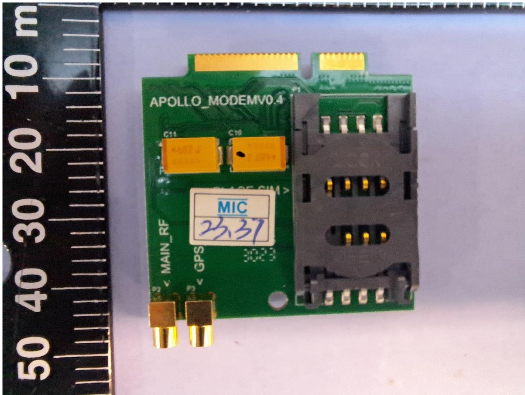
PCB with RF module, bottom view
